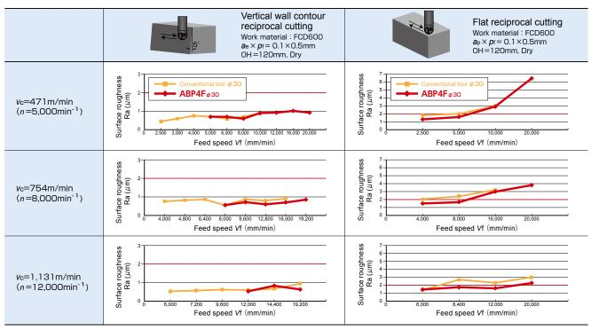
Note When Ra≤2µm is set as the standard, the test results shown above satisfy the standard when cutting vertical walls.
