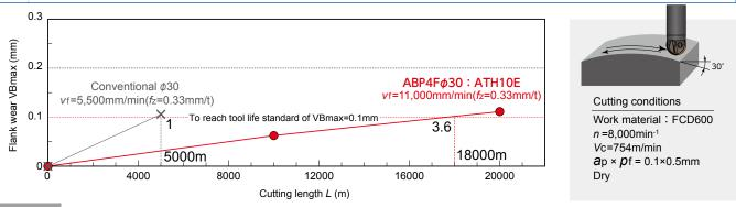
Conclusion Compared to conventional products, provides twice the cutting efficiency. 3.6 times the cutting length was achieved.
