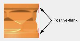
Although it is a double-sided specification, the flank is formed into a positive shape by the latest manufacturing technology and it achieves low cutting force.
