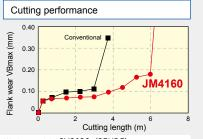
Work material: SUS630 (35HRC) Tool: AHU1532R-3 Insert: IDMT150508R
