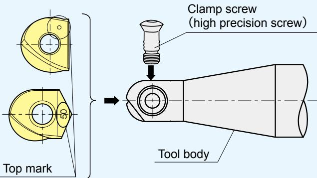
To meet the specification for precision of  $\pm 0.01\text{mm}$ , please follow this procedure.
